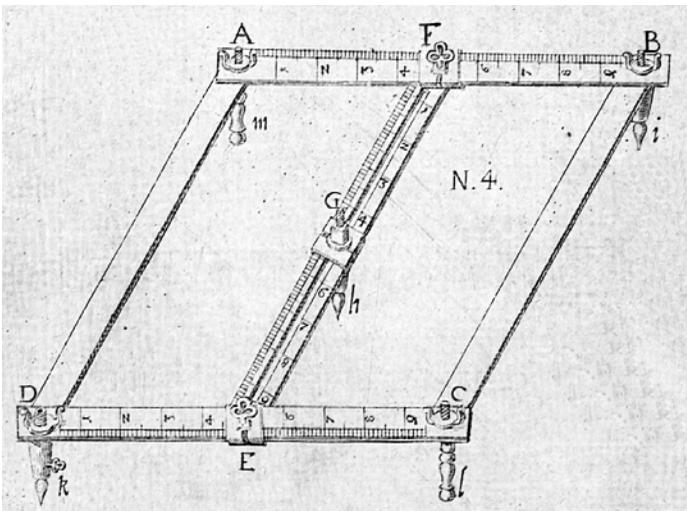
Abb. 23: Pantograph
